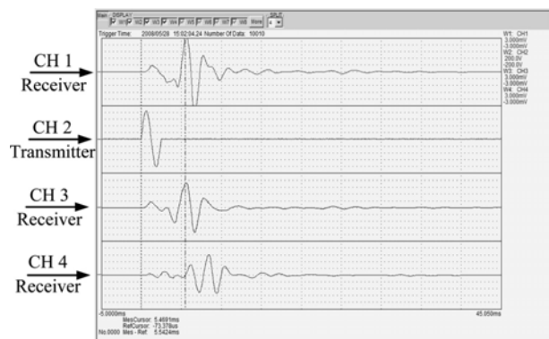
FIG. 8—Screen shot of the oscilloscope from a typical shear wave velocity measurement.
